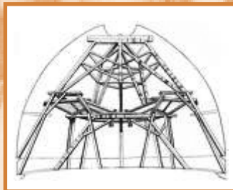
Dome Scaffold > in Florence Cathedral
